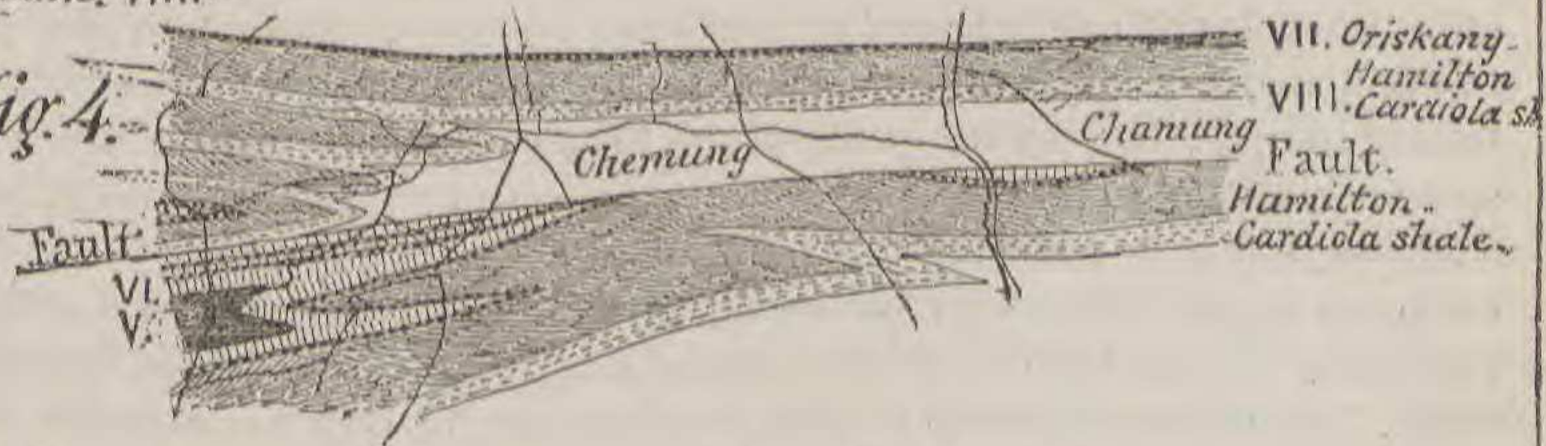
Fig. 1. Cross-section of the faulted district.
